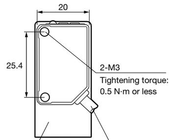
BEF-W100-B included with cable type  $\phi 3.8$ , 3-wire  $\times 0.2\text{m}^2$  (2-wire  $\times 0.2\text{mm}^2$  for through-beam type emitter)
